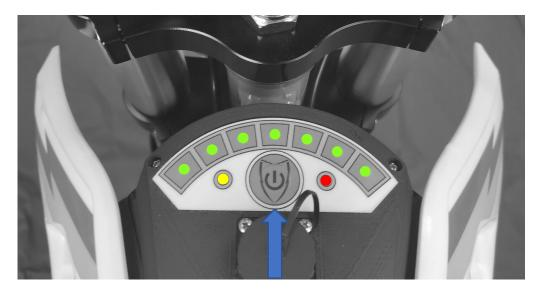
The on/off switch is in the middle of the display.
