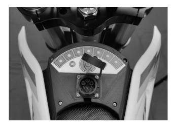
▷ Connect the charger's charging plug to the charging port of the motorcycle (bayonet closure), charging now starts automatically and the LED on the HVR charger lights up red.
