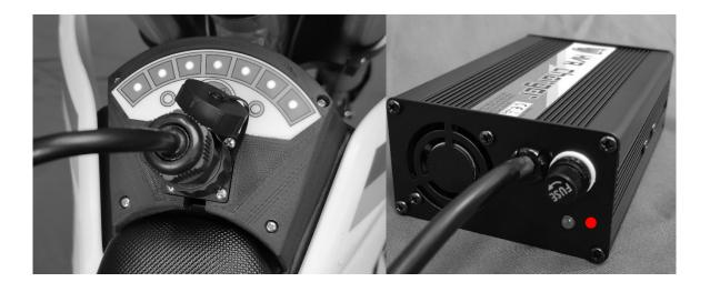
$\triangleright$  The flashing green LED on the motorcycle shows the current SOC.
